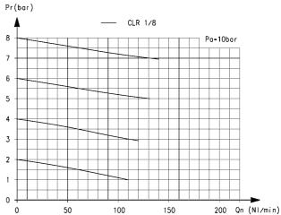
Pa = Inlet pressure (10 Bar) -Pr = Regulated pressure - Q = Flow CLR 1/4-6 6 bar  $\Delta P1 = 209$  NI/min CLR 1/4-8 6 bar  $\Delta$ P1 = 310 NI/min
