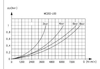
Flow diagram for model: MC202-L00
